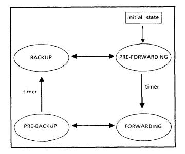
Upon startup, bridge B initializes each link to be in the PRE FORWARDING state, with the link database for each link initialized to claim B as the Root, B as the Designated Bridge on that link, B's distance from the Root to be 0, and the timer set to PRE\_FORWARDING\_DELAY.
