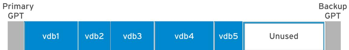
Figure 6.2: GPT Partitioning of the `/dev/vdb` storage device
